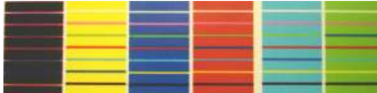
Figure 12 - Color bleed pattern showing easily observable color bleed
