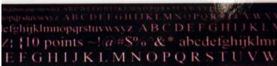
Figure 9 - Reverse text area after humidity exposure - ink bleed from black areas into white text
