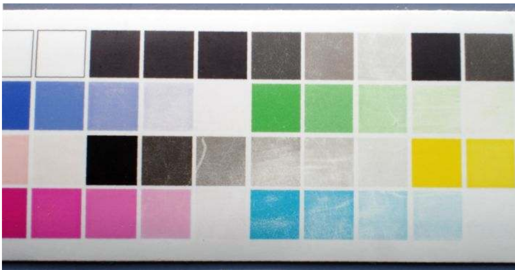
Figure 16 - Selective Fade on HP Kiosk after Gas Fade Exposure Test
