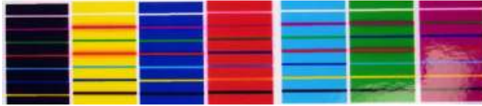
Figure 11 - Color bleed pattern showing easily observable color bleed
