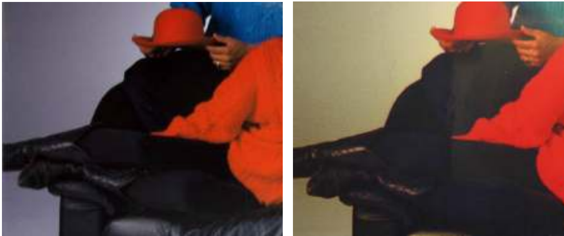
Figure 26 – Detail of sample before and after humidity exposure
