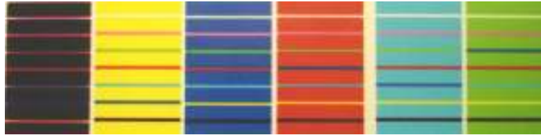
Figure 25 - Color bleed pattern showing easily observable color bleed
