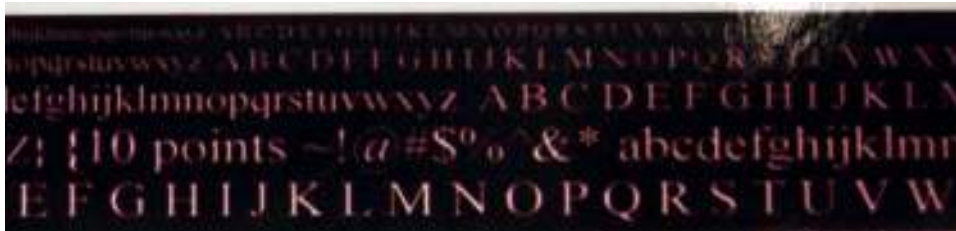
Figure 22 - Reverse text area after humidity exposure - ink bleed from black areas into white text
