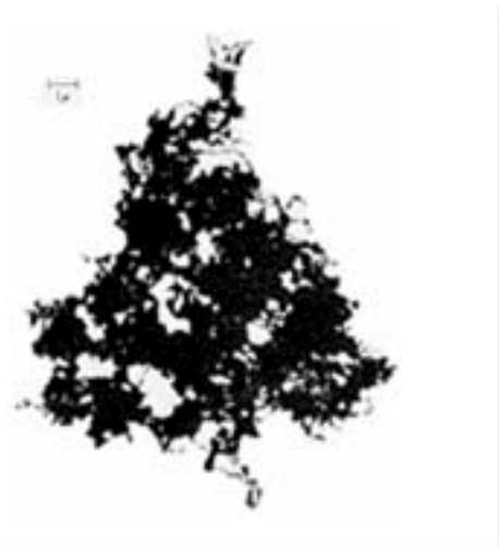
Figure 1b: An exposed silver halide crystal reduced by developer, thus forming much larger filaments of metallic silver.
