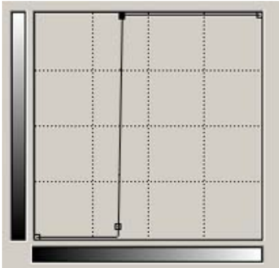
Figure 2a: Image line trace simulating a “sharp” edge from printer Dmax to paper white.
